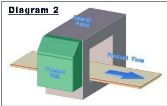
The ratio of the aperture size to the size of the product is important, to achieve optimum performance. The sensitivity of the detector is measured at the geometric centre of the aperture, which is the least sensitive point. This is inversely proportional to the size of the aperture - in particular, to the smaller of the two sides.
