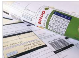
Printing barcodes and numbering in a defined space, including micro-printing for small text requirements to 3pt text and option to print at 1200dpi.
