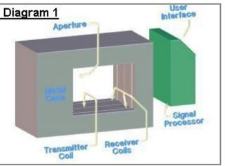
should select a metal detector which has been designed specifically for your application" As you will see in diagram 1, the typical detector is encased in a metal box. This houses the coil components, and provides a shield to protect them. The aperture - the tunnel through which the products pass - is lined with a non-metallic material (usually plastic), which provides an hygienic
